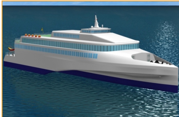
Three body high speed passenger transport ship
