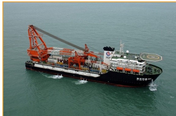
Large deepwater pipe-laying ship
