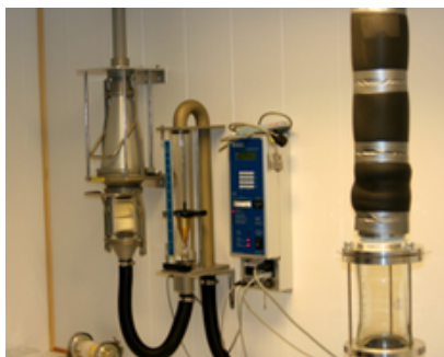
Air sampling equipment at the Zeppelin Observatory, Ny-Ålesund – long-term monitoring of pollutants in the Arctic. Photo: R. Kallenborn
